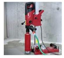
Use tool equipped with integrated water delivery None system that supplies water to cutting surface
